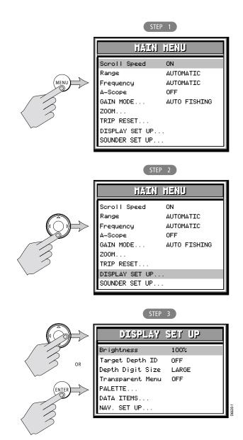
Figure 5-1: Accessing Display Set Up Menu Items
